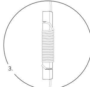
PLEASE NOTE! Always check if the cord is securely clamped inside bottom and top slit in the wooden pen (figure 3).
