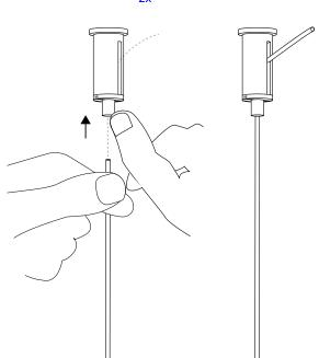
With all four cord-ends gripped inside the holders (fixed in the lamp) lift the lamp and fix the 2 vertical cord-ends inside the 2 ceiling attachments.
